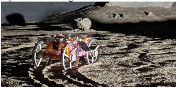
Figure 1: Development model of CubeRover in Mission Control's Moonyard undergoing integration and operations testing with Spacefarer™.
